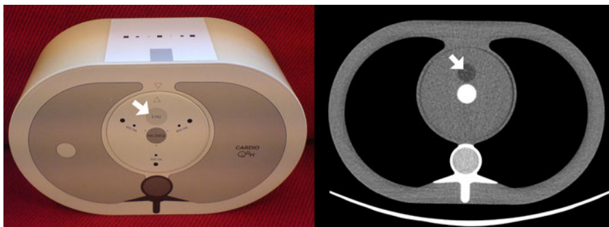
Fig. 3 The photograph (left) and CT image (right) of the thorax phantom
