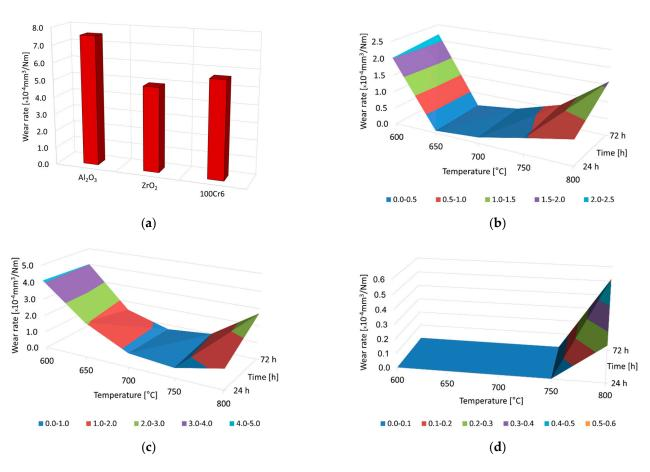
**Figure 5.** Wear rate for the Ti-6Al-7Nb alloy in the as-received condition (**a**) and after thermal oxidation at 600 °C, 650 °C, 700 °C, 750 °C, and 800 °C for 24 h and 72 h, after tribological tests with  $Al_2O_3$  (**b**),  $ZrO_2$  (**c**) and 100Cr6 (**d**) balls.
