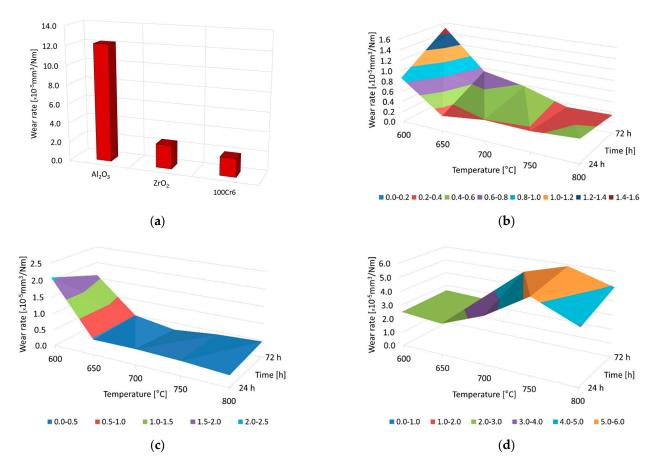
**Figure 6.** Wear rate of  $Al_2O_3$ ,  $ZrO_{2,}$  and 100Cr6 balls after tribological interaction with the Ti-6Al-7Nb alloy in non-oxidized (a) and oxidized conditions (b— $Al_2O_3$ ; c— $ZrO_2$ ; d—100Cr6) at  $600 \,^{\circ}$ C,  $650 \,^{\circ}$ C,  $700 \,^{\circ}$ C,  $750 \,^{\circ}$ C and  $800 \,^{\circ}$ C over a period of 24 h and 72 h.
