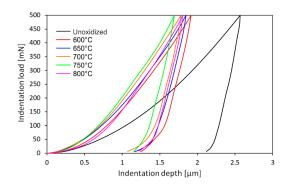
**Figure 4.** The constant peak-load of 500 mN for Ti-6Al-7Nb alloy, in the non-oxidized state and after oxidation at:  $600 \,^{\circ}\text{C}$ ,  $650 \,^{\circ}\text{C}$ ,  $700 \,^{\circ}\text{C}$ ,  $750 \,^{\circ}\text{C}$ , and  $800 \,^{\circ}\text{C}$  (72 h).
