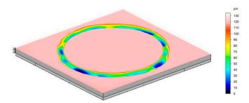
**Figure 10.** Corrugation wear on non-oxidized Ti-6Al-7Nb alloy disc, after tribological tests with 100Cr6 bearing steel balls.
