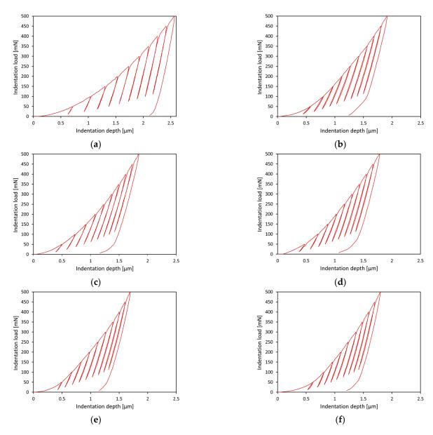
**Figure 2.** Representative indentation load-depth curves for the Ti-6Al-7Nb alloy in the initial state (a) and after oxidation at 600 °C (b), 650 °C (c), 700 °C (d), 750 °C (e), and 800 °C (f) over a period of 72 h.
