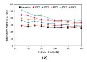
**Figure 3.** Hardness  $H_{IT}$  (**a**) and indentation modulus  $E_{IT}$  (**b**) of the Ti-6Al-7Nb alloy, depending on the oxidation temperature and indenter load.
