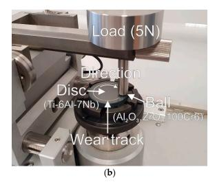
Figure 1. TRN tribometer: (a) general view, (b) detailed view of the tribological system.
