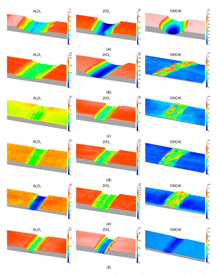
**Figure 9.** The 3D isometric images of the wear traces formed on the Ti-6Al-7Nb alloy surface after friction contact with  $Al_2O_3$ ,  $ZrO_2$ , and 100Cr6 balls ((a)—non-oxidized condition, (b)— $600\,^{\circ}C/72$  h, (c)— $650\,^{\circ}C/72$  h, (d)— $700\,^{\circ}C/72$  h, (e)— $750\,^{\circ}C/72$  h, (f)— $800\,^{\circ}C/72$  h).
