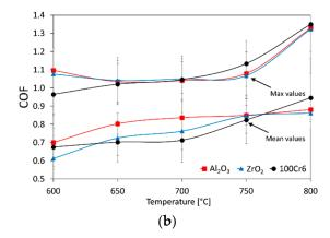
**Figure 8.** The influence of temperature and the friction couple on the average and maximum coefficients of friction values for Ti-6Al-7Nb after oxidation for 24 h (a) and 72 h (b).
