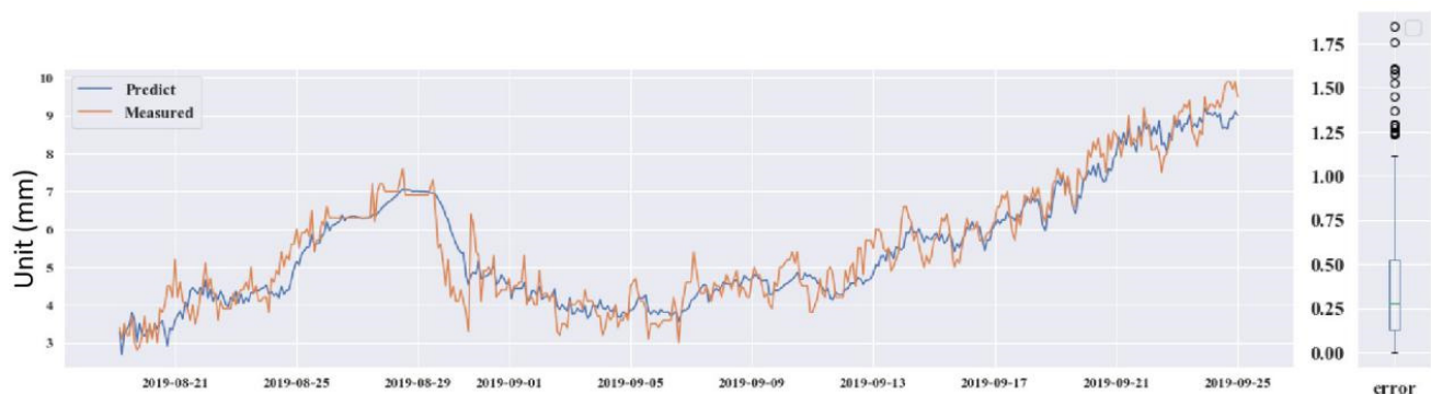
Figure 15. Predicted and measured planar displacement of GPS 12.
