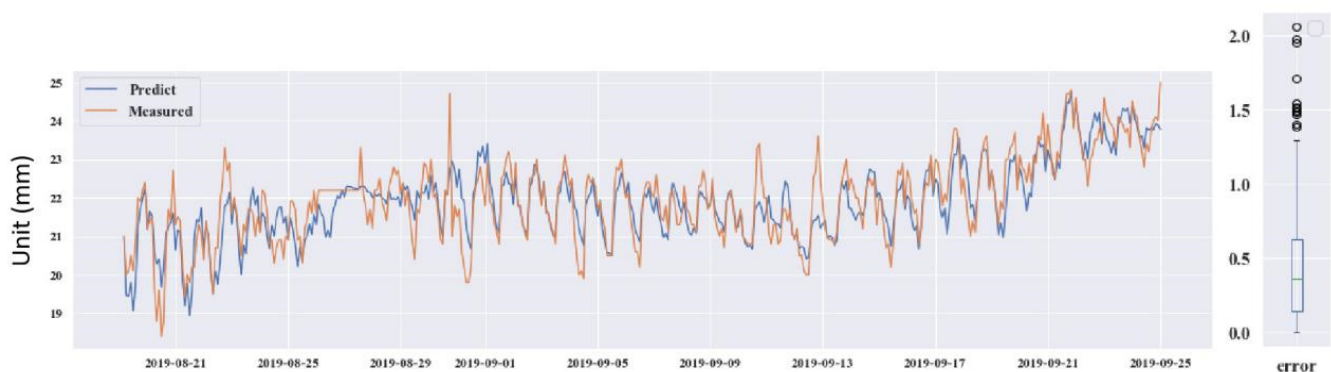
Figure 16. Predicted and measured planar displacement of GPS 14.
