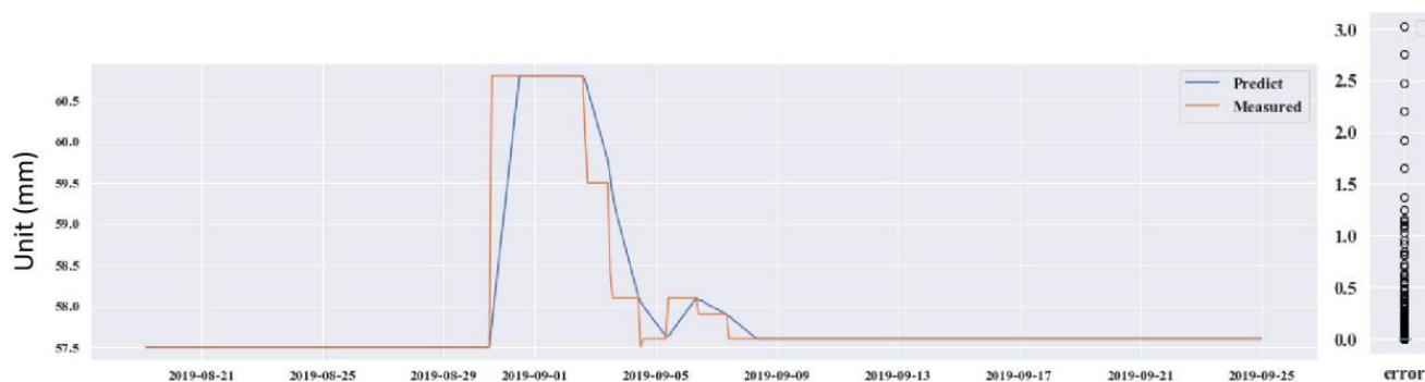
Figure 13. Predicted and measured planar displacement of GPS 04.
