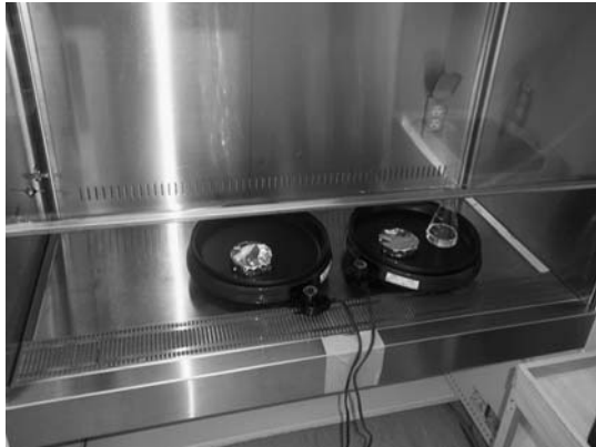
Fig. 12. Positioning of hotplates and sealing biosafety cabinets in preparation for fumigation
