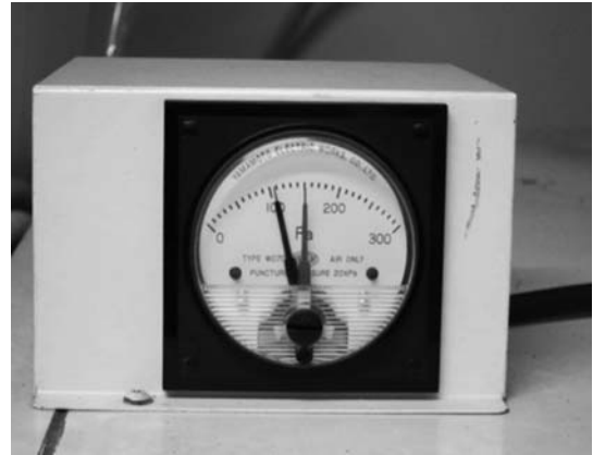
Fig. 9. Manometer of intermediate filter
