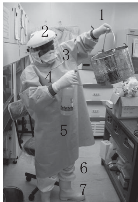
Fig. 6. P3 Lab user in full PPEs. 1: Gloves (double), 2: Face Shield, 3: N95 mask, 4: Wrist band, 5: Front covered gown, 6: Coverall, 7: Safety boots
