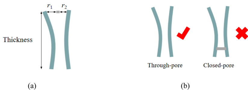
Figure 15. Side view of the pore morphology: (a) divided-pore and (b) through-pore and closed-pore.
