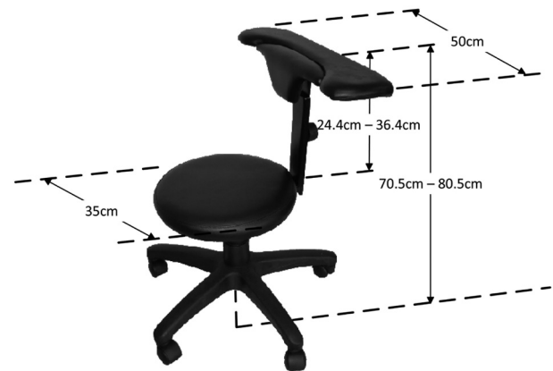
Fig. 1. The proposed chair with a height-adjustable seat and a back support, which can alternatively be used as an arm support.
