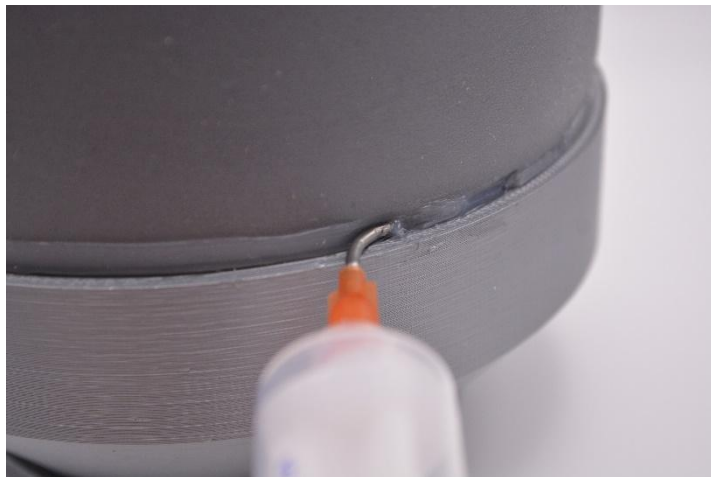
Fig. S2. The bottom dome of the Roliner is sealed using again Silpoxy glue. The glue was applied using a blunt-end bent syringe while the dome is pressure fitted into the reconfigurable composite.
