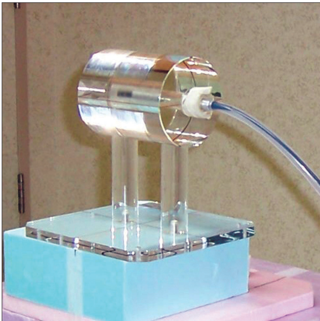
Figure 1: The cylindrical test tool to provide a constant depth of 5 cm for an FC65 ion chamber. Three angulations of the gantry can be checked with this tool routinely. Under-table gantry position cannot be measured as the mounting block comes in the path of the beam
