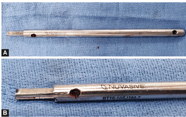
Figs 5A and B: Images of the distal portion of the broken PRECICE bone transport system with a 5 × 5 mm hole made using a high-speed carbide burr on the anterior aspect of the nail proximal to its lubricating cannister. Zoomed-out (A) and zoomed-in (B) views of the distal nail
