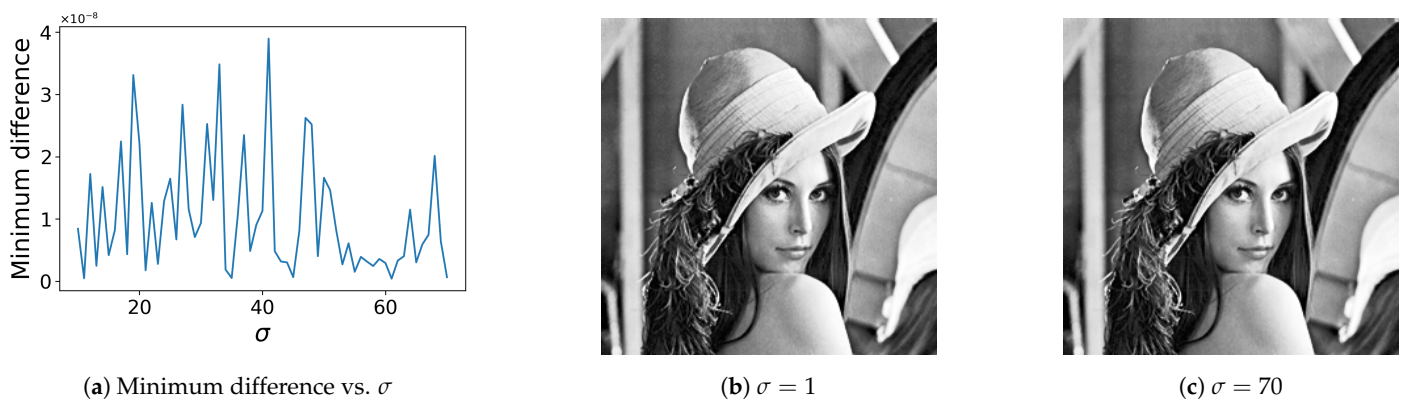
Figure 11. Insensitivity to parameter \sigma : (a) the minimum difference in the sorted values of F^{GF} as a function of \sigma . The positive values mean that there are no pixels with the same pixel value in Gaussian-filtered image F^{GF} , from which we have a strict ordering; (b) histogram equalization with \sigma = 1 ; (c) histogram equalization with \sigma = 70 .
