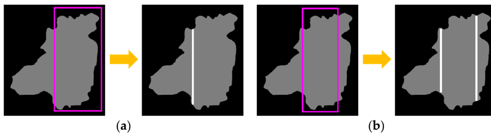
Figure 7. Segmentation with a single useful BB: (a) single boundary line; (b) two boundary lines.
