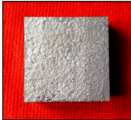
Figure 2. Stir casted AA8079 + TiN + ZrO 2 samples.
