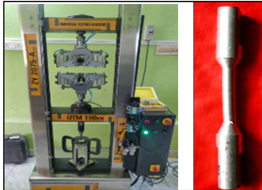
Figure 3. Schematic view of 100 kN capacity of UTM with tensile test specimen.
