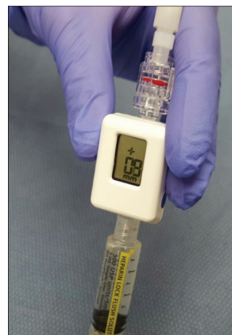
Figure 1. Compact manometer used for EUS-guided portal pressure measurement (Cook Medical, Bloomington, IN)
