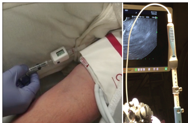
Figure 2. EUS-guided portal pressure measurement apparatus showing noncompressible tubing attached to the FNA needle inlet (right pane) and compact manometer being placed at the midaxillary line of the patient (left pane)
