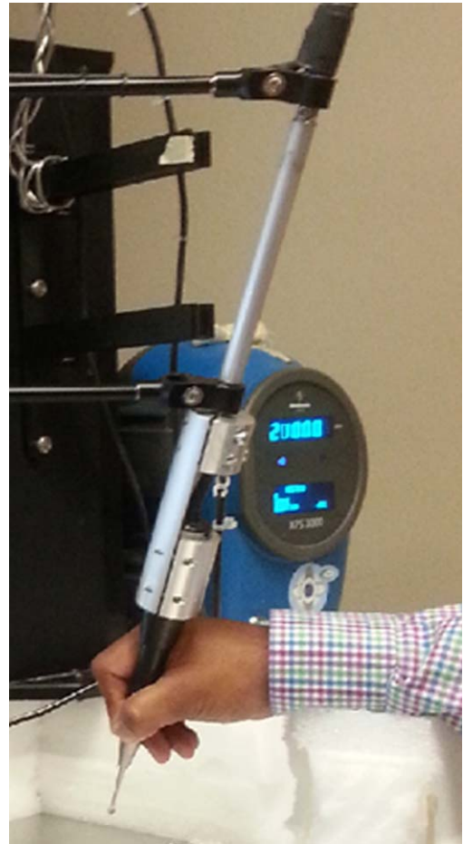
Fig. 3. Custom surgical drill gripper mechanism for HD 2 haptic device and polystyrene ergonomic support system. HD = high definition
