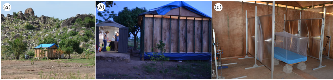
Figure 6. Field studies were undertaken at a rural location near Mwanza, Tanzania. (a) The experimental huts were erected approximately 500 m from known natural mosquito breeding sites, and from the nearest human and animal housing. (b) The small hut housed the recording unit from where the observer operated the cameras of the tracking system as they recorded mosquito activity in the large hut. (c) The complete tracking system showing the LEDs on the left, the paired Fresnel lenses on either side of the bed and bed net and cameras on the right.
