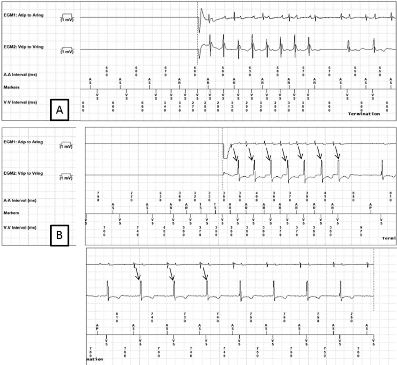
Fig. 1. Panel A: The ventricular channel (Vtip to Vring) shows ventricular sensing at a cycle length of 290 ms, and is dissociated from atrial activity on the atrial channel (Atip to Aring). Far field ventricular activation is visible on the atrial channel. This was classified as a true VHR episode. Panel B: The ventricular channel shows ventricular sensing at a cycle length of 360 ms. The atrial channel shows 1:1 atrioventricular activity, which persists after termination of the episode (thin black arrows). This was classified as a false VHR episode.
