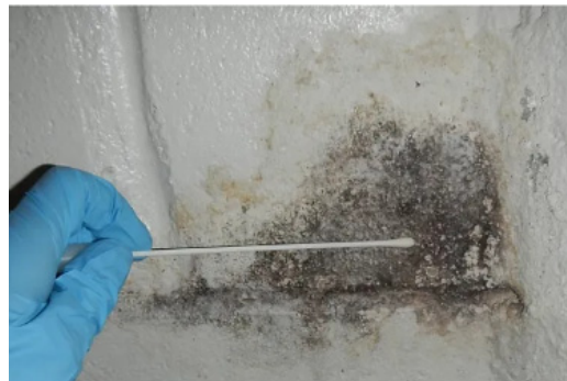
Figure 3. Moldy surface sampling using a sterile swab (template is not present on the photo).
