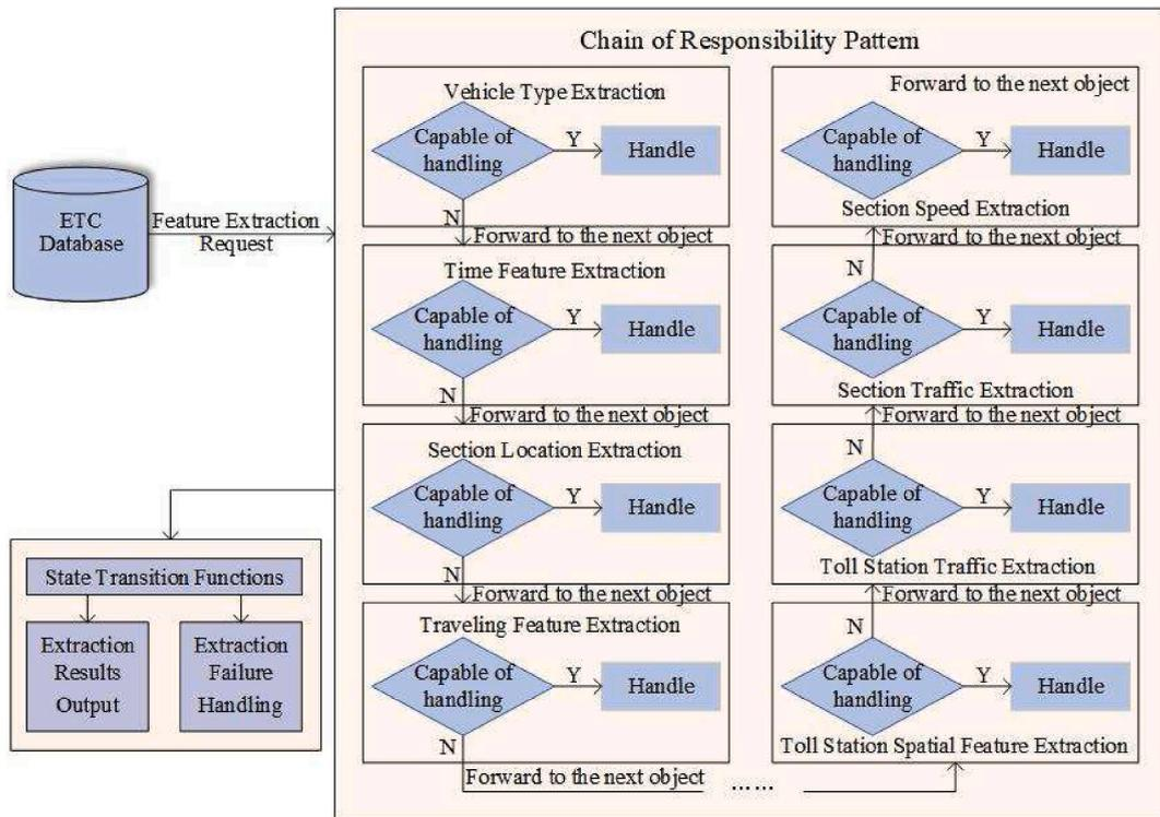
Fig. 2. Flowchart of feature extraction algorithm.
