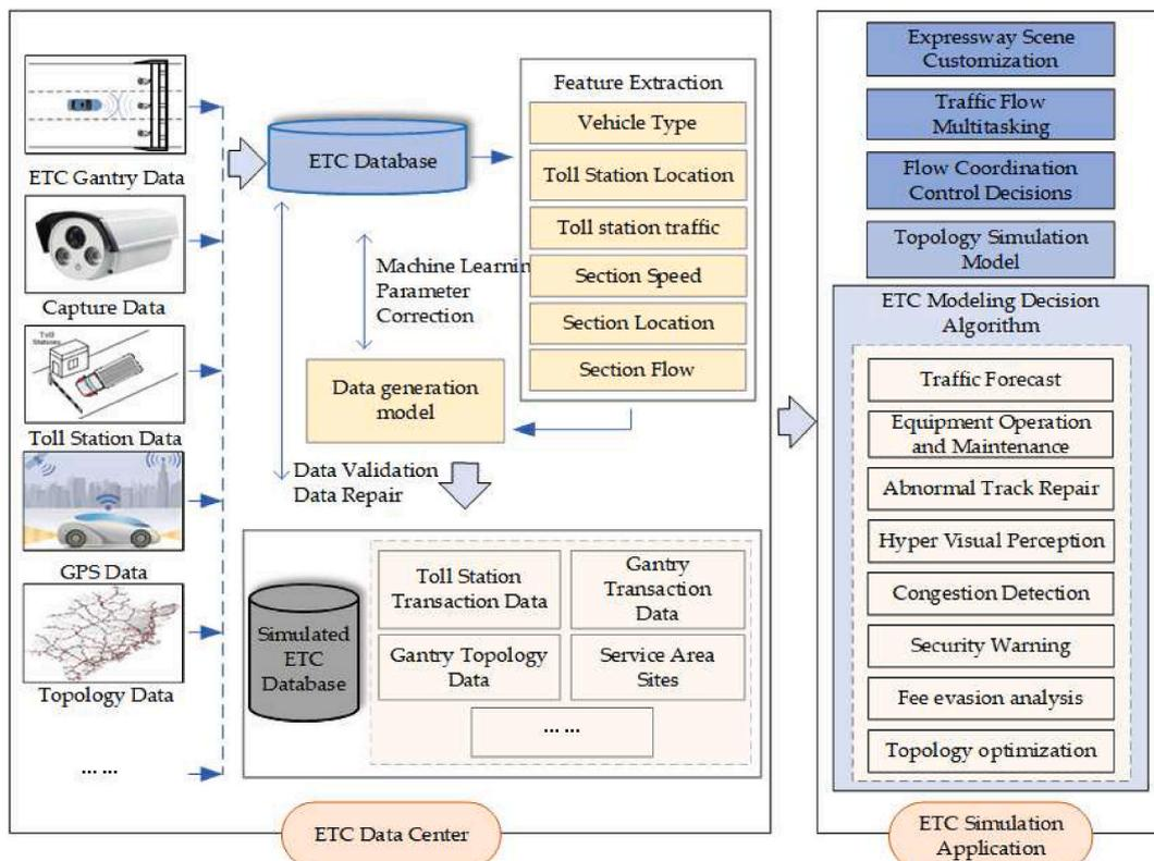
Fig. 1. Components of ETC simulation system of intelligent expressway.
