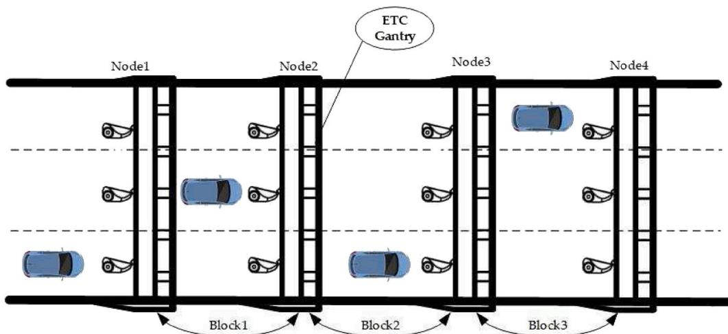
Fig. 3. Schematic diagram of Block.
