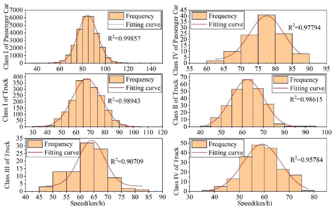
Fig. 9. Speed characteristics of some vehicle types in Block B.
