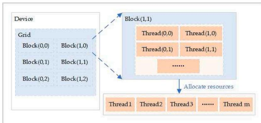
Fig. 4. The management structure of system’s threads.
