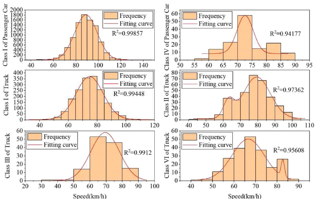
Fig. 8. Speed characteristics of some vehicle types in Block A.
