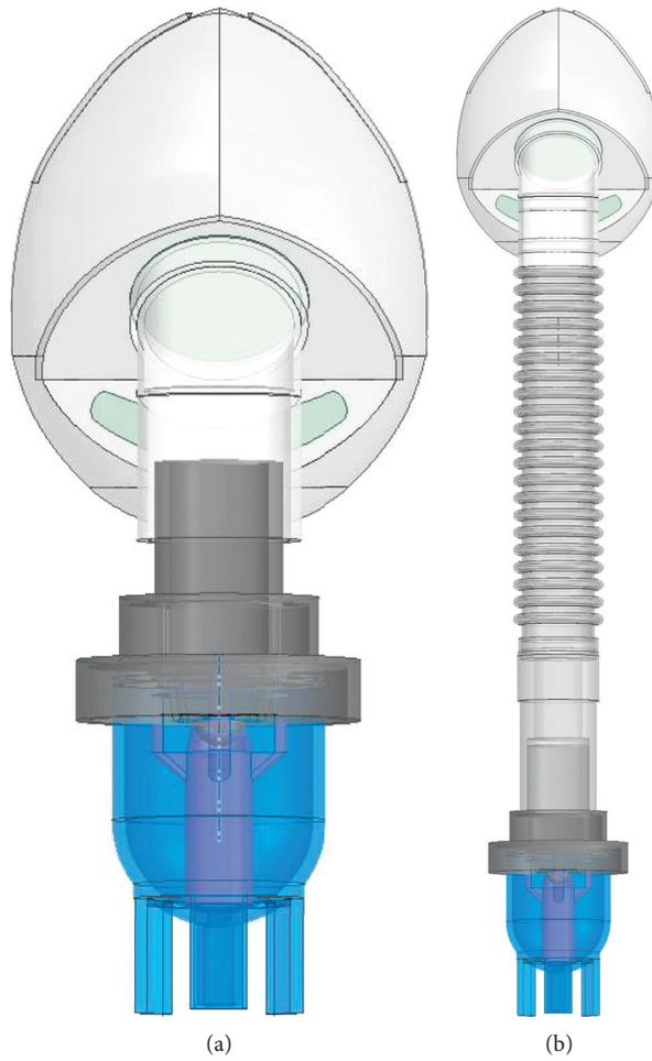
FIGURE 3: Solid models of (a) traditional and (b) modified SVJNs.
