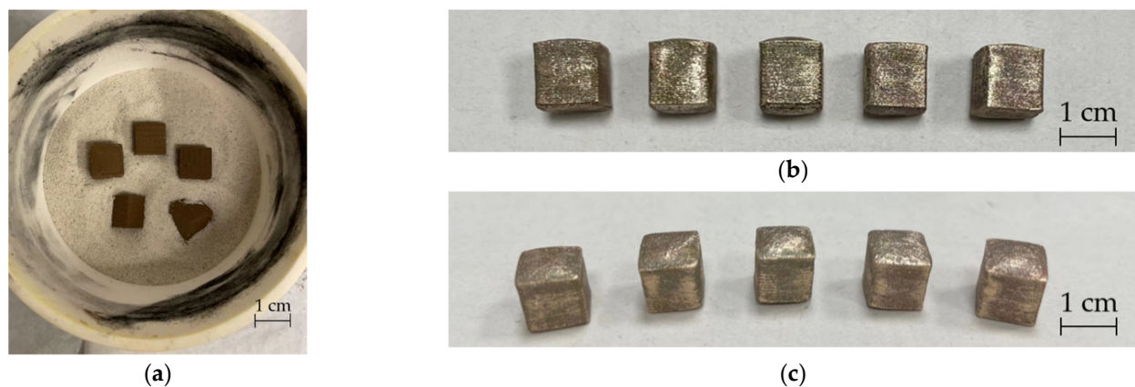
Figure 5. Sintered cubes according to five sintering directions before and after sintering: (a) cubes according to five sintering directions were embedded in sand; (b,c): cubes after sintering (from left to right: sintering on xy surface, on xz surface, on yz surface, on an edge, and on a point).
