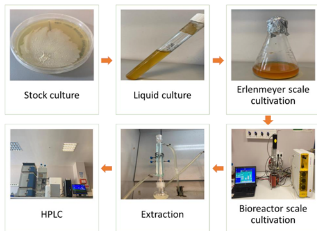
Fig. 5. A flow chart of obtaining squalene from Schizochytrium limacinum for cosmetic analyses (courtesy of the authors). HPLC: high pressure liquid chromatography.
