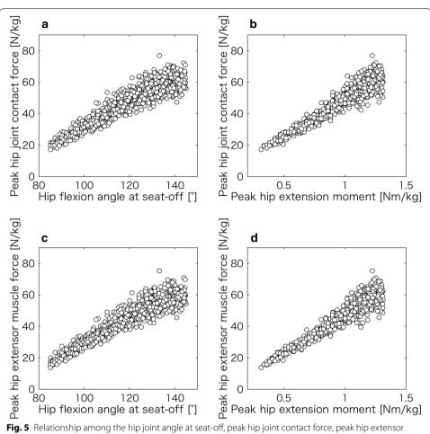
**Fig. 5** Relationship among the hip joint angle at seat-off, peak hip joint contact force, peak hip extensor muscle force, and peak hip extension moment during the STS movements. All relationships in **a–d** are approximately linear
