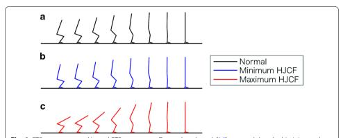
**Fig. 6** STS movements. **a** Normal STS movement. Doorenbosch et al. [16] reported that the hip joint angle at seat-off is  $93.4 \pm 8.4^\circ$ . Thus, the STS movement when the hip flexion angle at seat-off is closest to  $93^\circ$  is regarded as a normal STS movement (black solid line). **b**, **c** STS movement when the hip joint contact forces are minimum (blue solid line) and maximum (red solid line), respectively
