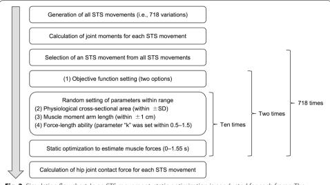
**Fig. 2** Simulation flowchart. In an STS movement, static optimization is conducted for each frame. The muscle forces during an STS movement are estimated 20 times by using variable parameters. Therefore, estimations of muscle forces were conducted  $14,360 \ (= 20 \times 718)$  times in this computer simulation study
