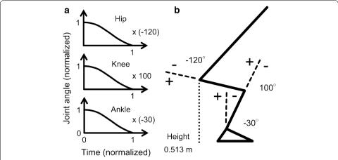
**Fig. 4** Illustration of **a** normalized joint angles and **b** a posture at seat-off. The normalized joint angles of the hip, knee, and ankle joints are multiplied by the hip, knee, and ankle angles at seat-off, respectively, to generate an STS movement
