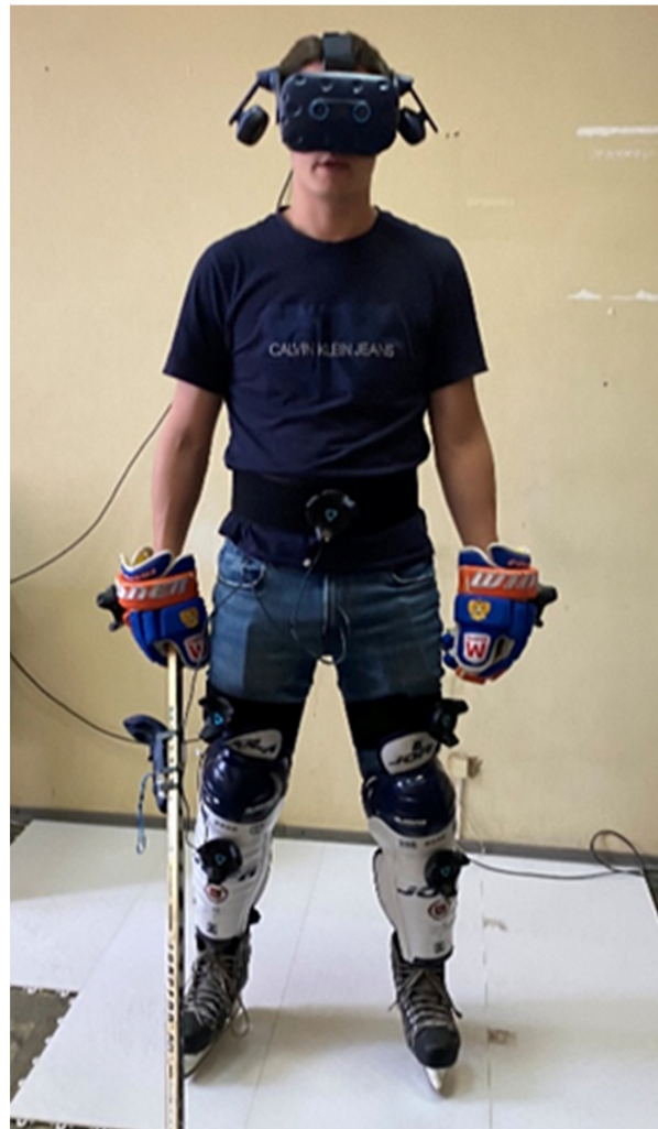
Figure 4. Subject with the trackers attached to his shin guards, hips, chest, gloves and stick.
