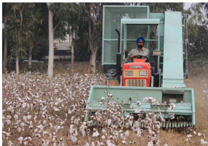
Fig. 7. Tractor operated cotton stripper [52].
