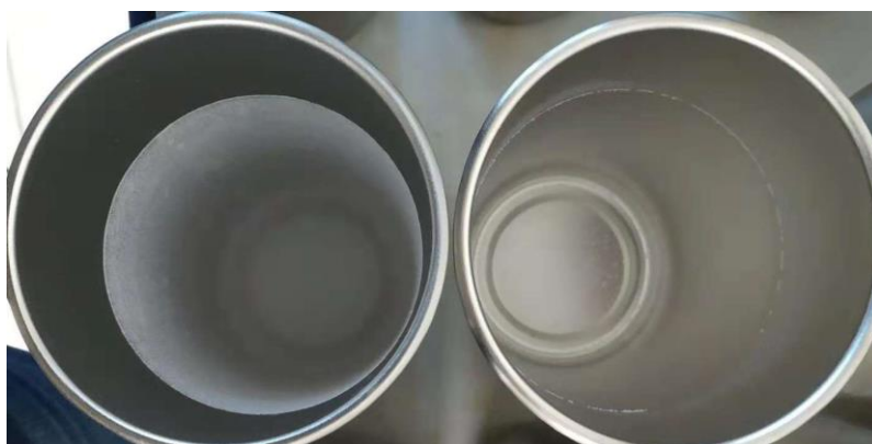
Figure 4. The image of the \text{CaCO}_3 scales attached to the experimental cup in the absence of an inhibitor (left) and in the presence of 100 mg/L carbon nanoparticles (right).
