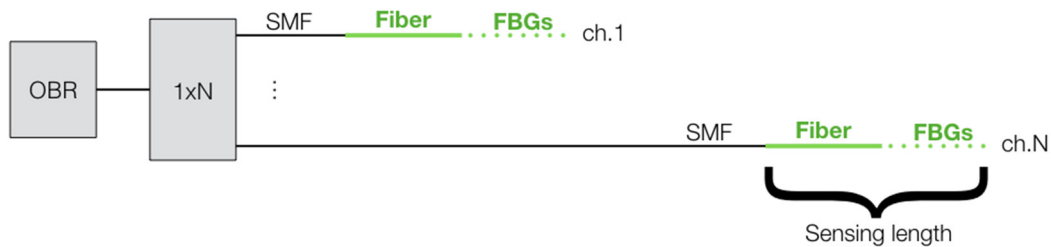
Figure 9. Sketch of the range-extended operation of SLMux through Fiber Bragg Gratings (FBGs).
