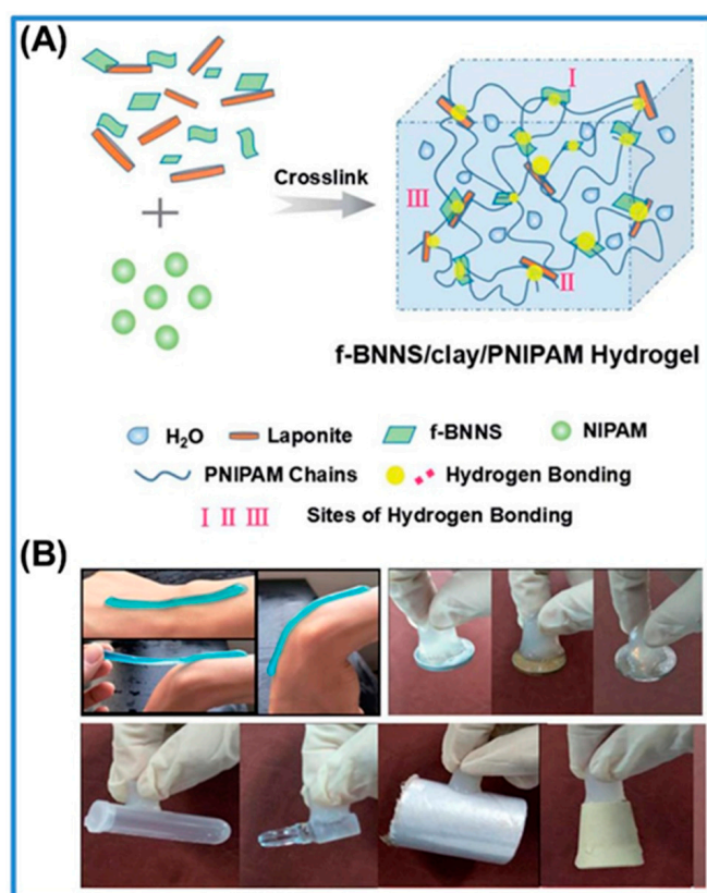
Figure 5. (A) Schematic illustration of the formation of the f-BNNS/clay/PNIPAM ternary network hydrogel. (B) Hydrogel adhesion on the arm, aluminum, copper, iron, plastics, glasses, polythene and rubbers. Adapted with permission from Ref. [133]. Copyright (2018) The Royal Society of Chemistry.
