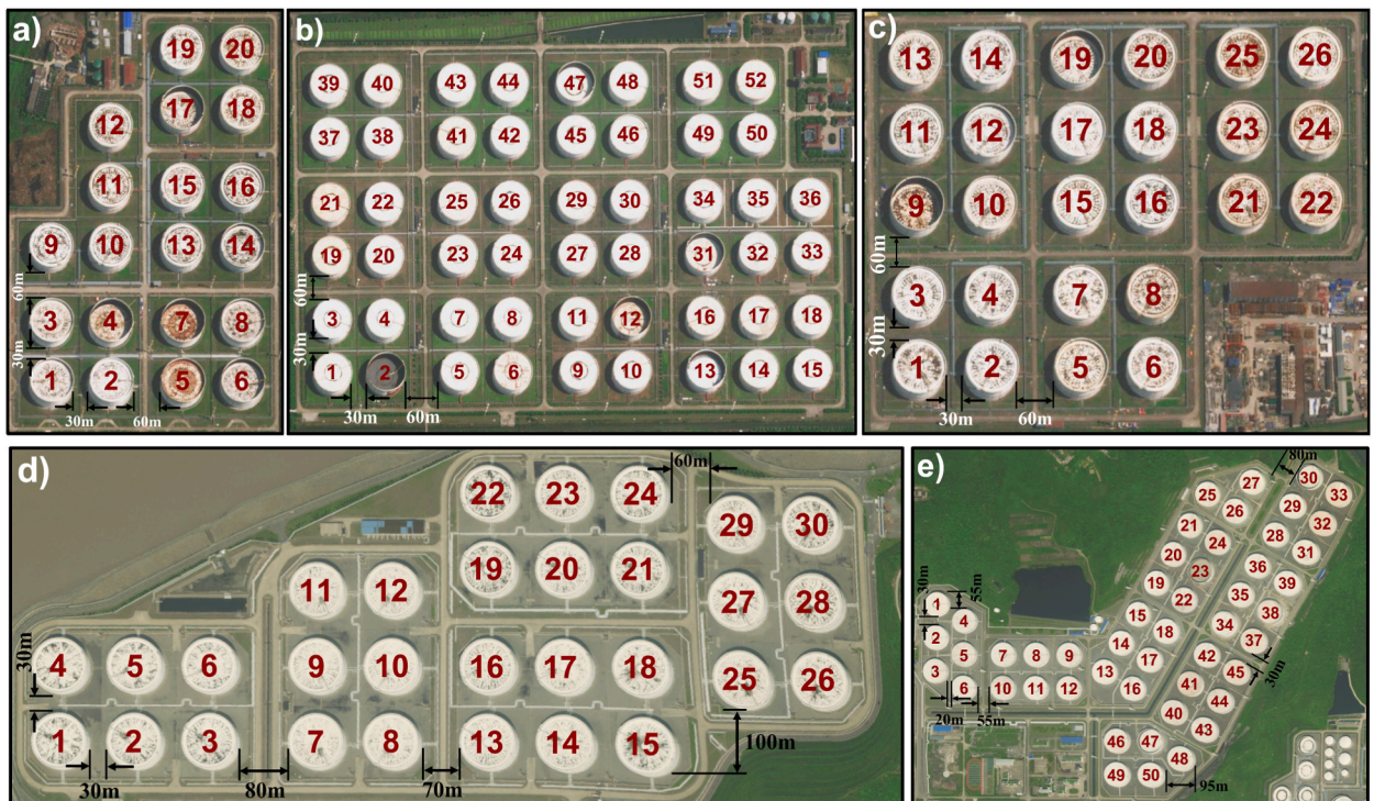
Fig. 4. Layouts of five existing storage plants: (a) Plant 1, (b) Plant 2, (c) Plant 3, (d) Plant 4, and (e) Plant 5.
