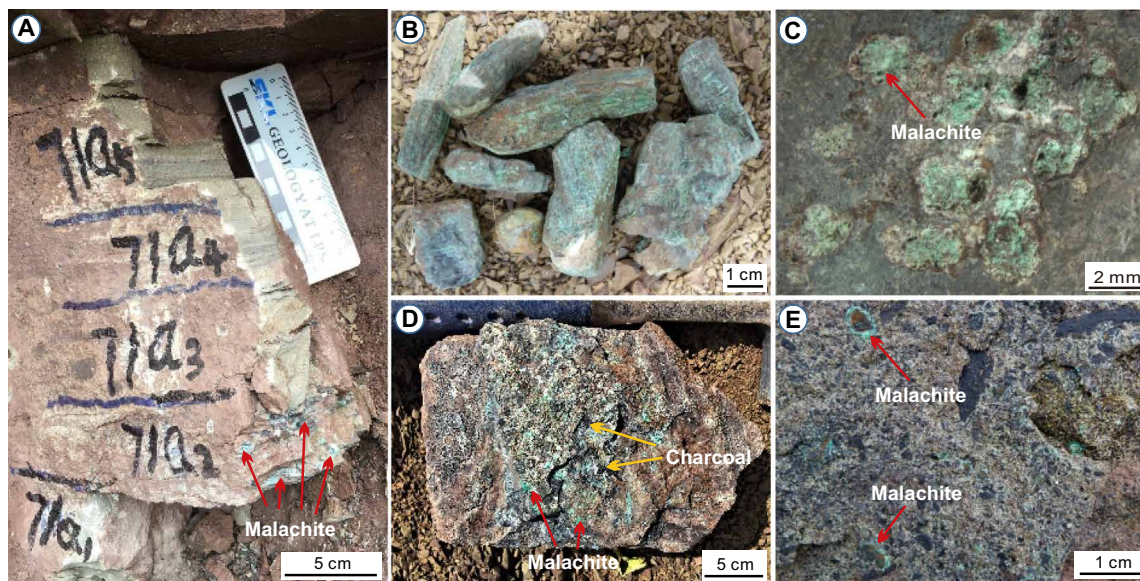
Fig. 1. Photographs and photomicrographs of the Cu-rich sulfide and charcoal from the terrestrial Permian-Triassic transition. (A) Rock sample from TSJ-71a, TSJ section; (B) rock sample LB-16 from LB section; (C) rock sample from GBC-3b-3, GBC section; (D) rock sample of bed TSJ-71a with malachite and charcoal from TSJ section; and (E) rock sample of bed LMD-38-2 with malachite from LMD section. Photo credit: H. Zhang, Nanjing Institute of Geology and Palaeontology.
