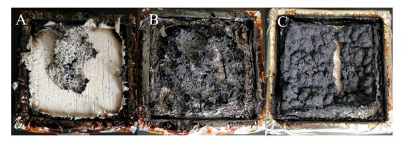
Figure 4. Digital images of char residue obtained from cone calorimeter test: (A) TAD0; (B) TAD12; and (C) TAD6EG6.
