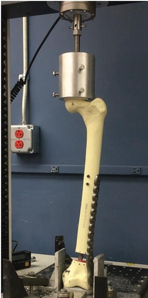
**Figure 3.** Axial loading setup. The femur is secured proximally in a custom acetabular cup and distally on a polyethylene tibial insert. The specimen is loaded along the femoral mechanical axis. The distal fragment is set between 2 blocks, preventing coronal and sagittal translation of the distal segment during axial loading.
