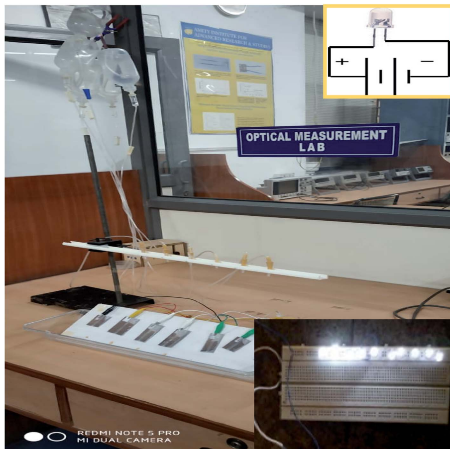
Fig. 4 A photographic and circuit-based representation of MPA-HEG powering 10–12 commercial LEDs.
