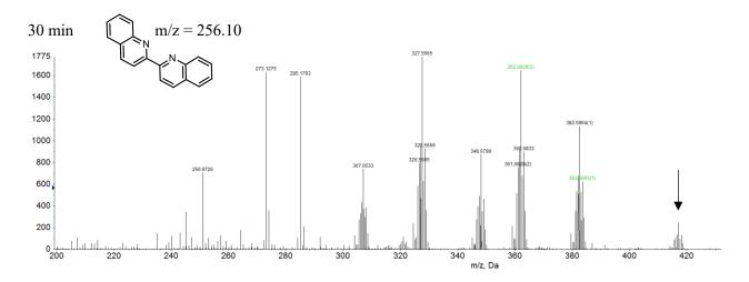
Rubiq (5 mM in  $H_2O$ ) and exposed to 617 nm light (10 mW/cm<sup>2</sup>) with constant mixing. Samples were removed at 5, 10, and 30 min and analyzed by ESI-MS. Significantly, the mass peak for the monosubstituted product,  $Ru(biq)_2(4$ -azidobutyronitrile)( $H_2O$ ), 370.58 was not observed, rather the fully substituted product  $Ru(biq)_2(H_2O)_2$  was observed even at the shortest light exposures.
