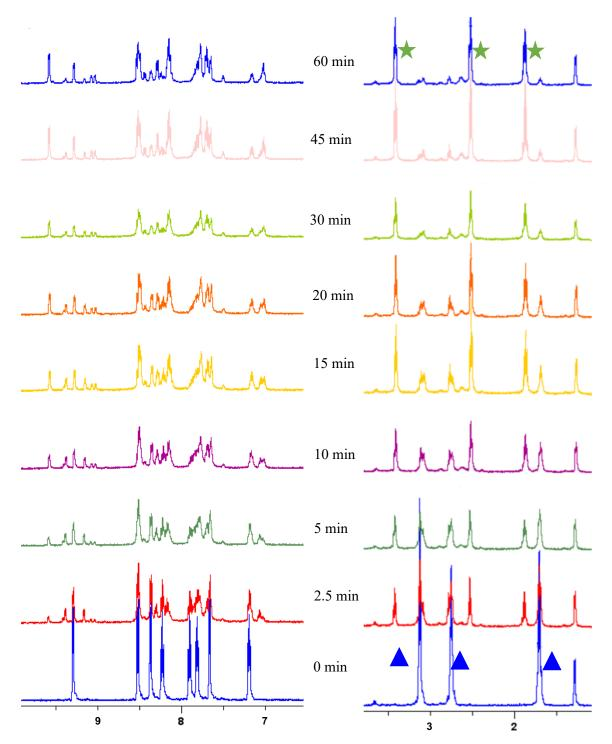
Rubpy (5 mM in  $D_2O$ ) and exposed to 530 nm light (7.8 mW/cm<sup>2</sup>) with constant mixing. The sample was probed by  $^1H$  NMR at various time points to determine intermediate photolysis products. The complete loss of peaks corresponding to coordinated 4-azidobutyronitrile (blue triangle, 1.70, 2.75, and 3.13 ppm) and increase of a new set of peaks (green star, 1.87, 2.52, 3.41 ppm) indicates exchange of both azide-bearing ligands beginning in the first minutes of irradiation.
