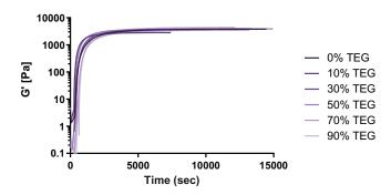
In situ rheometric analysis of hydrogel formation with equal ratios of all three photolabile crosslinkers (i.e., Rubiq, Rubpy, and oNB) and increasing amounts of nondegradable diazido-tri(ethylene glycol) (TEG) crosslinker (0 – 90%). Studies performed in the dark.
