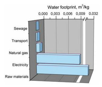
Figure 11. Main components of production system generating water footprint of glass fibers.
