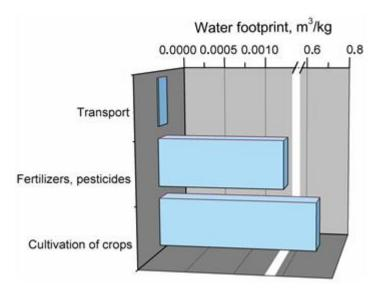
Figure 10. Main components of production system generating water footprint of kenaf fibers.
