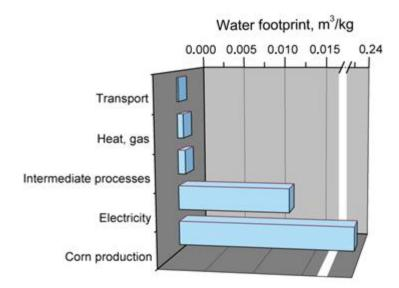
Figure 7. Main components of production system generating water footprint of poly(lactic acid).
