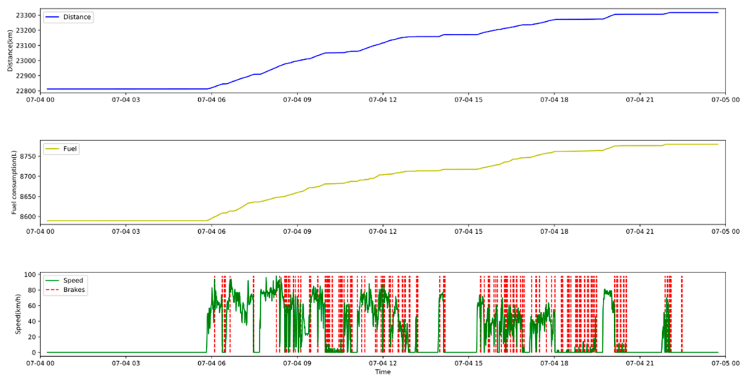
Figure 2. Distance covered, fuel consumption, speed and braking of a vehicle in the course of one day.
