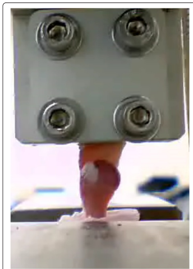
Figure 3 Biomechanical testing. Supraspinatus tendon-humerus specimen was mounted on a material testing system by using a specially designed jig.
