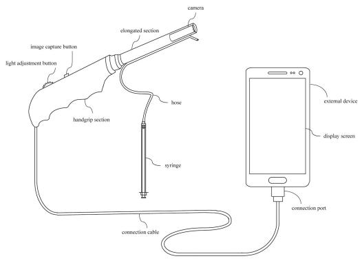
Fig 6. Citobot 1.0, cervical cancer early detection device, system, and method.
