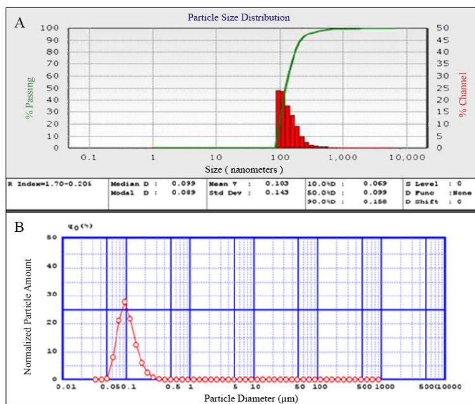
Fig. 1. (A) Dynamic light scattering and (B) particle size analyzer graphs of artemether-loaded nanostructured lipid carriers with average diameter of 103 nm.
