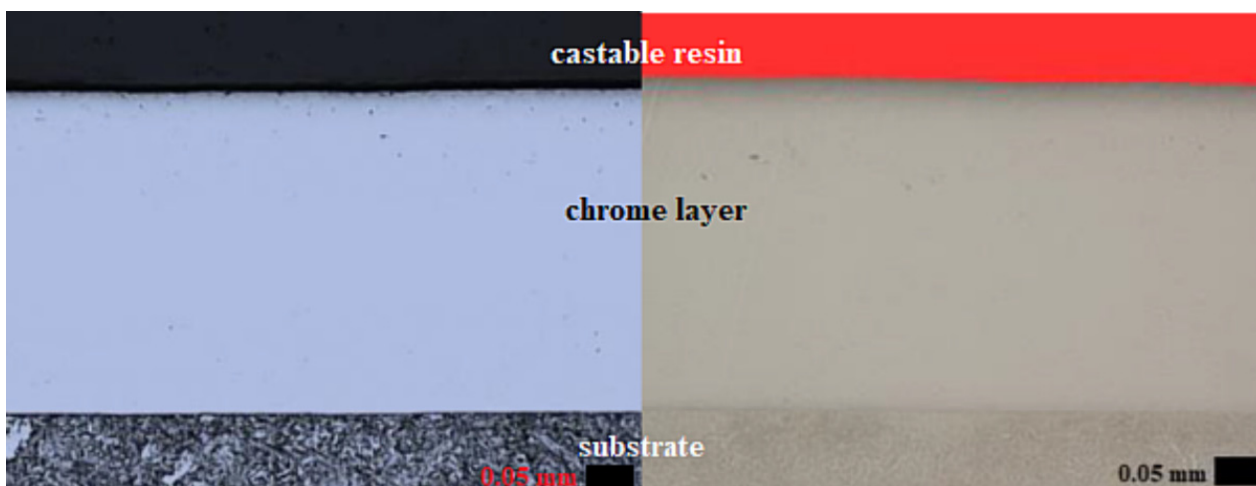
Figure 2. The microstructure and porosity of uncut sample (sample 0).
