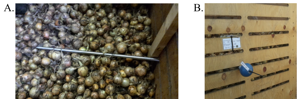
Fig 1. Placement of the Hortisens spear in a two-ton box with onions. Inside view of the box at the time of filling with middle sensor 8 cm away from the tip and edge sensor next to the wooden side of the box (A). Outside view with transmitter (blue ball) and black antenna (B). Photos: Jacob Skov Pedersen, Technological Institute.
