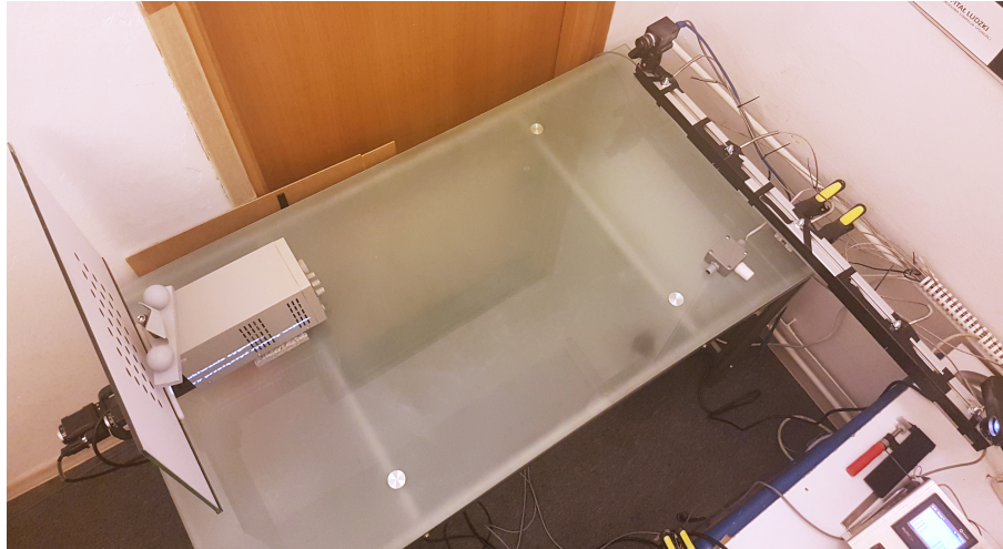
Figure 15. The test stand used in the verification experiments. The 3D-structured light scanner is equipped with a set of heating resistors that can heat its mechanical base. Six temperature sensors measure the temperature of the base. In the measurement volume of the scanner, there is a ball-bar for validation and a calibration artifact in the background.
