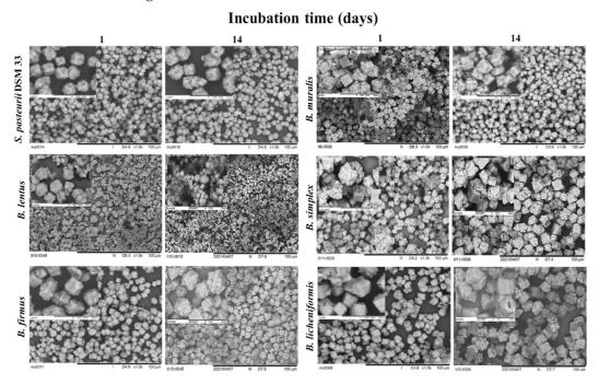
**Figure 10.** Low magnification SEM images ( $1000 \times$ ) and their corresponding higher magnification as an inset in the left upper corner ( $5000 \times$ ) for the obtained precipitates.
