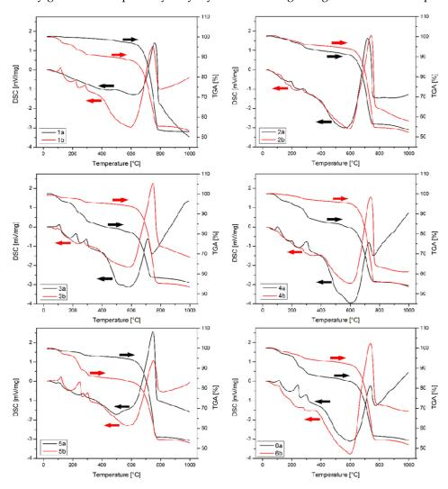
**Figure 9.** DTA/TGA of CaCO<sub>3</sub> precipitates (a—1st day; b—14th day; 1—*S. pasteurii* DSM 33; 2—*B. muralis*; 3—*B. lentus*; 4—*B. simplex*; 5—*B. firmus*; 6—*B. licheniformis*; black arrow—1st day; red arrow—14th day).
