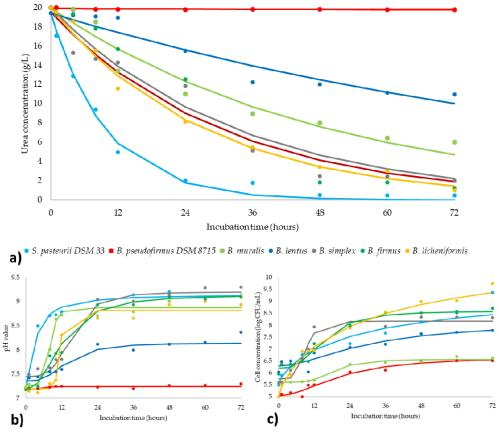
**Figure 4.** Kinetic study of (a) ureolysis process; (b) pH value; (c) bacteria concentration (markers signify the experimental data; lines indicate predictive results).
