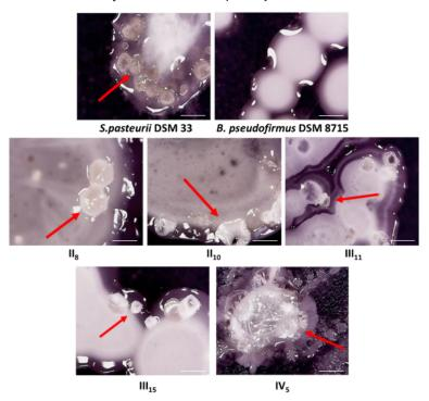
**Figure 2.** Optical microscopy of bacterial colonies on Urea-CaCl<sub>2</sub> agar ( $400 \times \text{magnifications}$ ; scale bar 2 mm; red arrow indicated crystal formation with different positions relative to the colony center).
