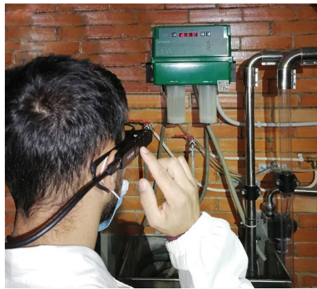
Figure 5. Operator with SG while accessing the maintenance augmented instructions through the QR code (40 mm), placed on the milking machine management control unit (green box).
