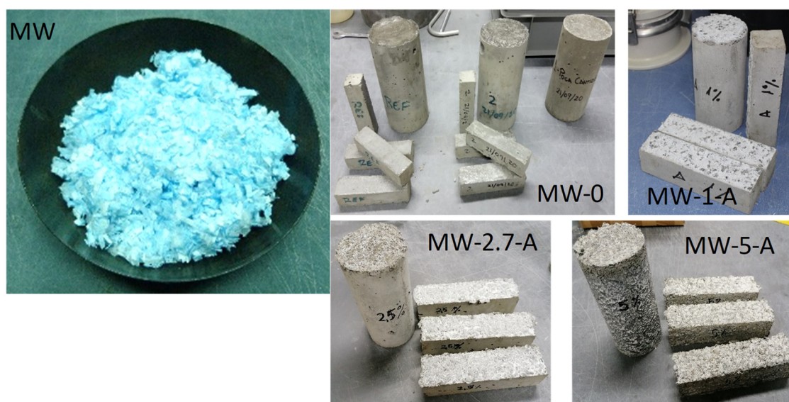
Figure 1. Shredded MW ready to be included in the mortar, and aspect of some of the mixes.
