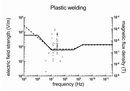
Fig. 1. Maximum electric field strength (left y-axis) and magnetic flux density (right y-axis) at the worker's position per publication, per main frequency component for dielectric heating of plastic.
