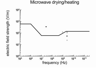
Fig. 5. Maximum electric field strength at the worker's position per publication, per main frequency component for industrial drying or heating processes. Legend: — = electric field strength action levels; ● = electric field strength. Symbols in grey represent data published before 2012 and symbols in black data published in or after 2012. Literature references used: <sup>40, 88–91</sup>
