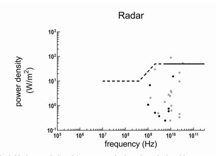
Fig. 6. Maximum equivalent plain wave power density at the worker's position per publication, per main frequency component for radar devices.
