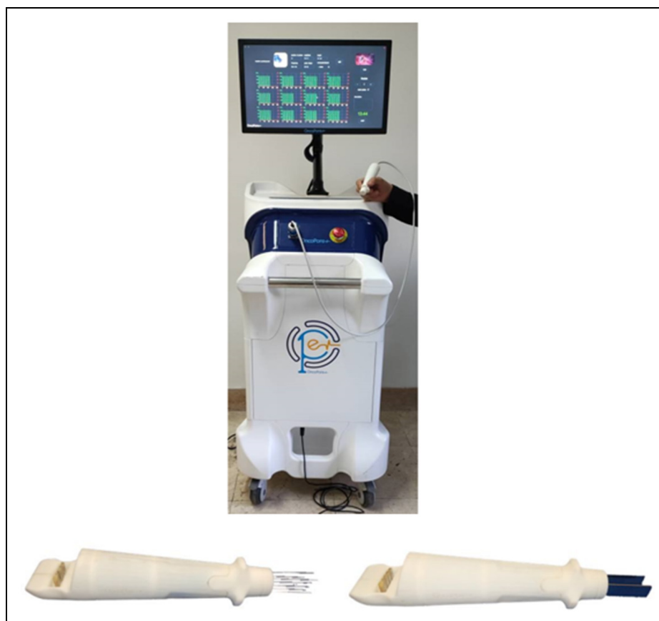
Figure 1. Up: Electroporation System (OncoPore, Iran). Hexagonal Needle (Bottom Left) and Double Parallel Plate (Bottom Right) Electrodes.
