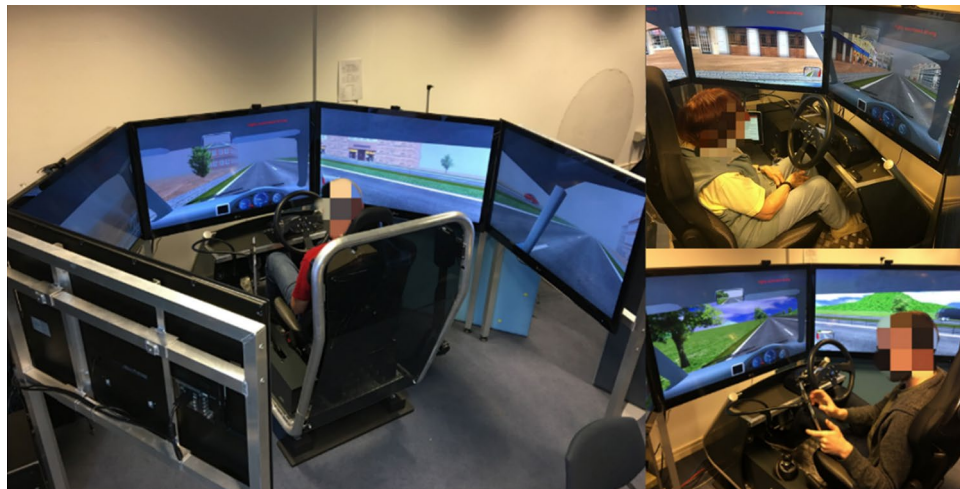
Figure 1. Newcastle University Fixed-based ST software Jentig50 driving simulator.
