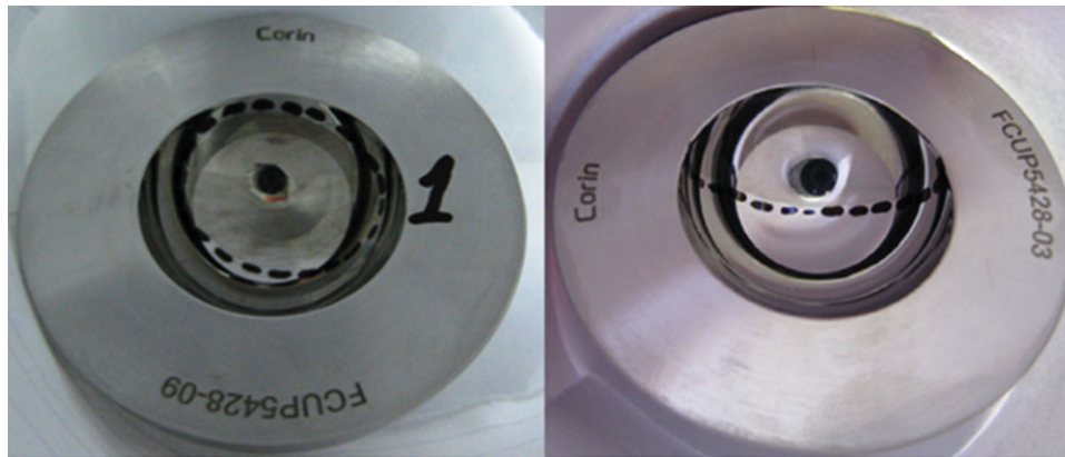
FIGURE 9. Photographs of the 28-mm inner diameter acetabular cups showing the wear area (within dotted line) under standard conditions with 45° inclination angle (left) and the wear area under steep inclination angle (right). Under steep inclination angle, the wear area intersected with the rim of the acetabular cup. [Color figure can be viewed in the online issue, which is available at wileyonlinelibrary.com .]
