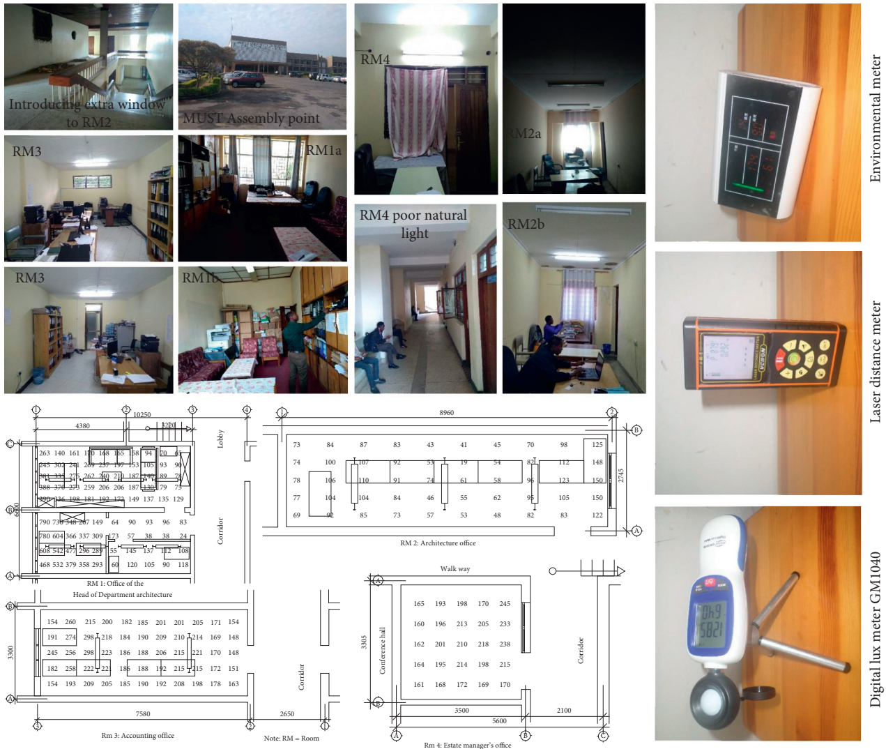
FIGURE 1: The floor plans of the representative offices and images showing the impression of lighting set up and the equipment involved in measurements.
