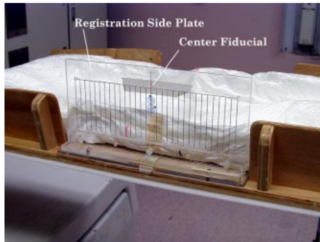
FIG. 3. (Color) Registration side plate mounted on carrier box.
